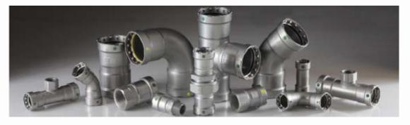
The State of Connecticut has approved the new Viega MegaPress system for applications for natural gas and propane gas. This system eliminates the need to thread pipe for black steel pipe gas installations. MegaPress is for gas piping 1/2" through 2" with working pressures up to 125PSI. It also has a fitting for chilled water, compressed air, hydronics and low pressure steam under 15PSI.
